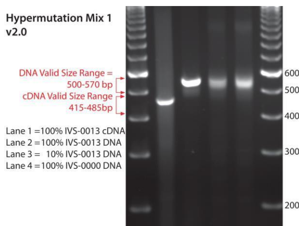
Figure 2. Amplified products were generated using Hypermutation Mix 1 v2.0 then run on 2% Metaphor agarose/TBE gel.
